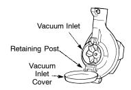
Place the hooks on the vacuum tube on the retaining posts; pivot tube into position. Secure vacuum tube by turning the knob clockwise until tight.
